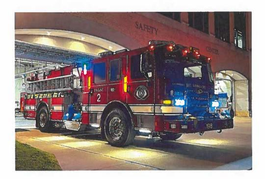
In 2023, the department placed into service a new Pierce Enforcer Class A Pumper, replacing a unit purchased in 2002. Ergonomically, the engine was designed to be easier to drive. It's lower to the ground and shorter in length, which allows it to make sharper turns. The engine holds 500 gallons of water, and large, brightly lit gauges on the back and both sides of the engine make it easy for firefighters to tell from a distance how much water is left.
