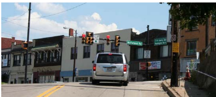
Pedestrian signal and crosswalk not visible to traffic (McFarland Rd. at Washington Rd.)
