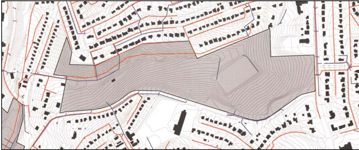
Diagram of the sub-surface infrastructure present in and around the park. Blue lines indicate storm sewers and red lines indicate sanitary sewers, which exist within and around the park.
